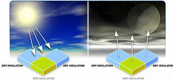
During the day the sun radiates energy, and heats up the roof.
