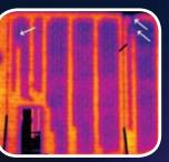
Infrared quality control testing of CMU wall construction.
