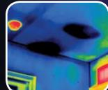
Locating moisture problems in buildings using infrared thermography.
